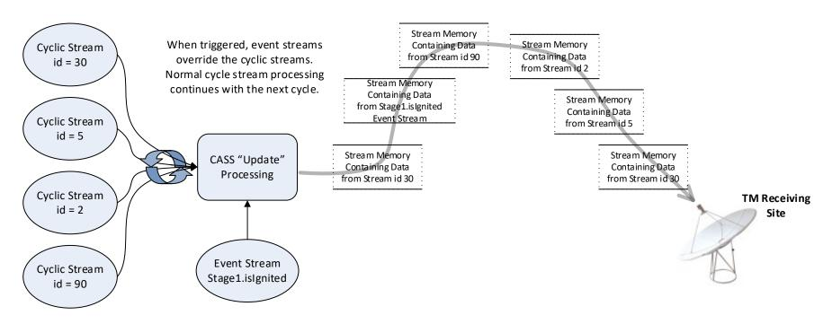
Streams allow the user to obtain information from the CASS flight software within the AFTU during testing and flight.
