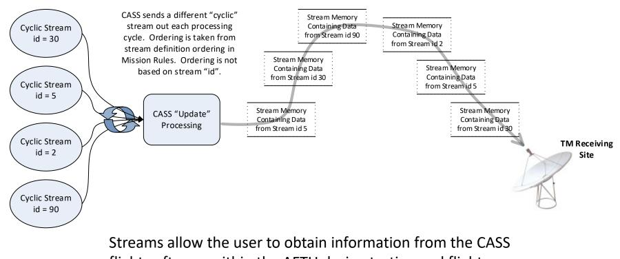
flight software within the AFTU during testing and flight.
